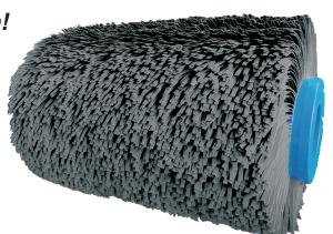
The abrasive grain silicon carbide black with a crystalline and sharpedged structure has a high hardness and brittleness. This results in a micro-splitting of the grain, which brings out new sharp edges. Particularly suitable for a beautiful and glossy surface.
