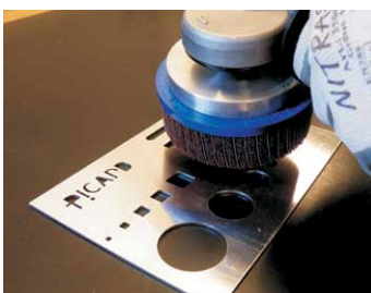
Deburring disc FAPI-M14 used on an angle grinder
