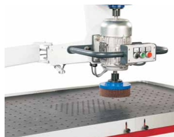
Deburring disc FAPI-150 used on a Manual Grinder from Timesavers B.V.
