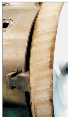
contact wheel core after the first turn off process
